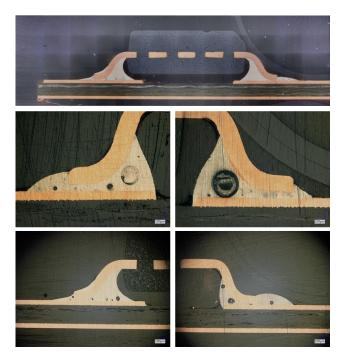
Fig. 17 Metallographic cross-sections of selected solder joints produced via induction soldering.
