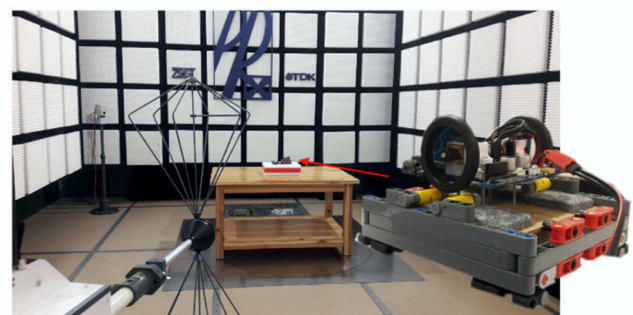
Fig. 4 Configuration of the measurement bench inside the anechoic chamber and the tested object along with the brake
