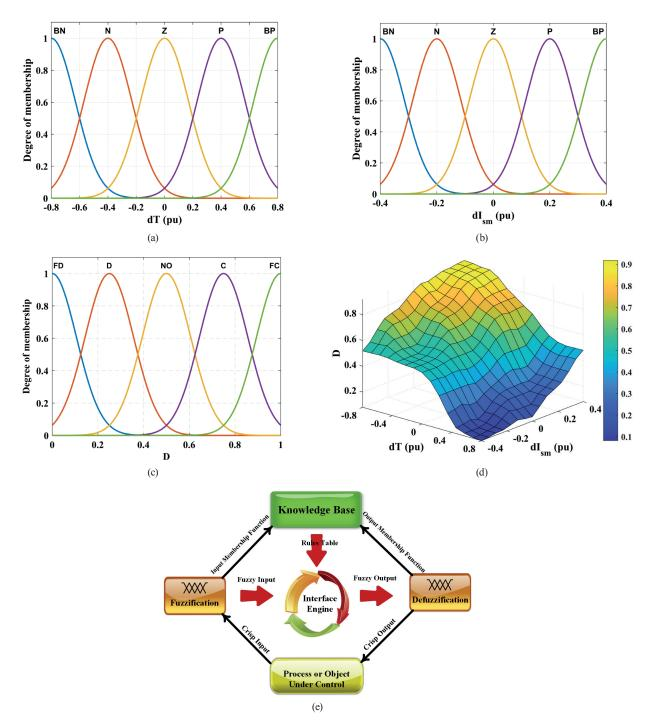
Fig. 6 Inputs and output variables of membership functions and FLC complete process. (a) Input 1 of MF, dT (pu), (b) Input 2 of MF, dIsm (pu), (c) The output of MF, (D), (d) The 3-D graph for inputs-output MFs, (e) Complete procedure of FLC. BP = Big positive, P = Positive, Z = Zero, N = Negative, BN = Big Negative, FC = Fast charging, C = Charging, NO = No action, D = Discharging, FD = Fast discharging.
