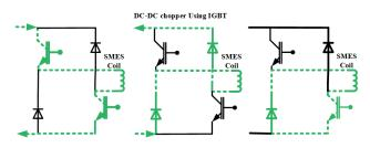
Fig. 5 Operation modes of the DC–DC chopper. (a) Charging mode, (b) Discharging mode, (c) Standby mode.
