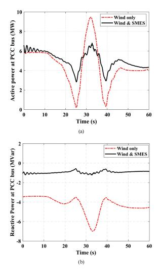
**Fig. 10** Response of line active and reactive powers at PCC bus. (a) Active power at PCC bus, (b) Reactive power at PCC.
