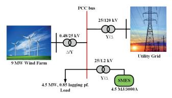
Fig. 2 Power system model under study
