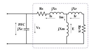
Fig. 1 Equivalent circuit of SCIG
