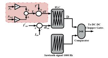
Fig. 4 FLC system for the chopper circuit
