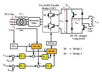
Fig. 3 Schematic diagram of VSC control SMES system
