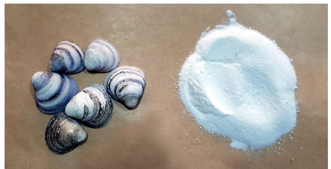
Fig. 3 River shells samples and their ground into powder form
