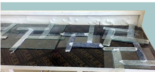
Fig. 5 Glass molds used in sample casting
