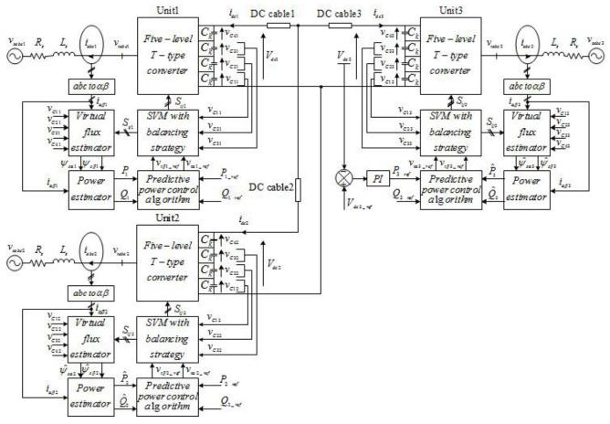
Fig. 1 Configuration of the proposed MTDC system
