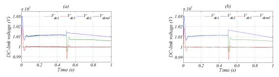
Fig. 8 Simulation results of DC-links voltages during converter disconnection: (a) with VF-DPC-SVM control (b) with VF-PDPC-SVM control
