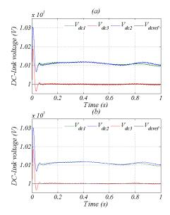
**Fig. 4** Simulation results of DC-links voltages: (a) with VF-DPC-SVM control, (b) with VF-PDPC-SVM control
