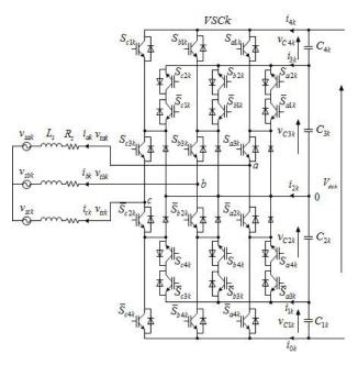
**Fig. 2** Main circuit of five-level T-type converter (k = 1, 2, 3)
