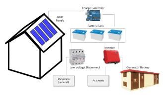
Fig. 2 Off-grid PV System
