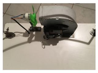
Fig. 6 Mini wind turbine with the inflow providing the source
