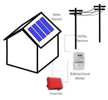
Fig. 1 Grid-connected PV System
