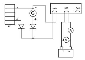
Fig. 5 Block diagram of university research station
