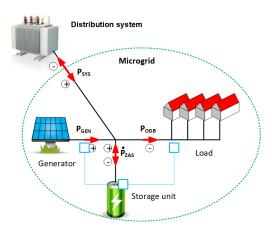
Fig. 3 Scheme of a microgrid [11]
