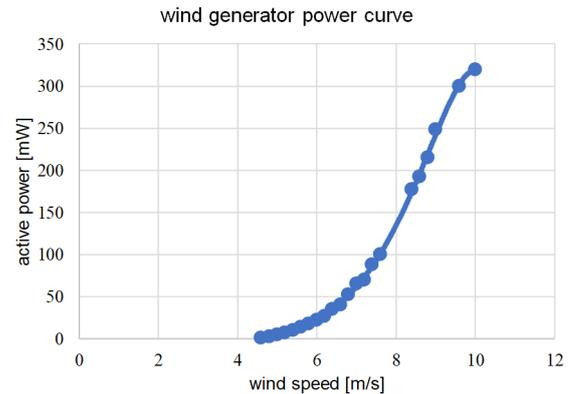
**Fig. 12** Wind generator power curve
