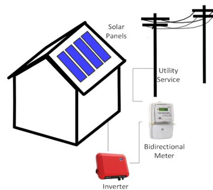
Fig. 1 Grid-connected PV System
