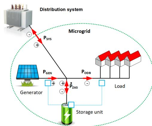
Fig. 3 Scheme of a microgrid [11]
