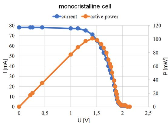
Fig. 9 Characteristic of monocrystalline cell
