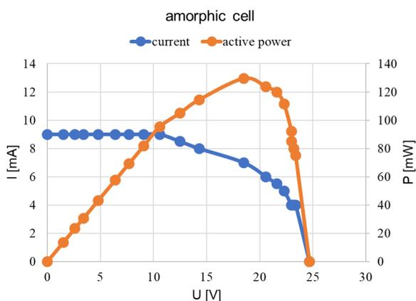
Fig. 8 Characteristic of amorphous cell
