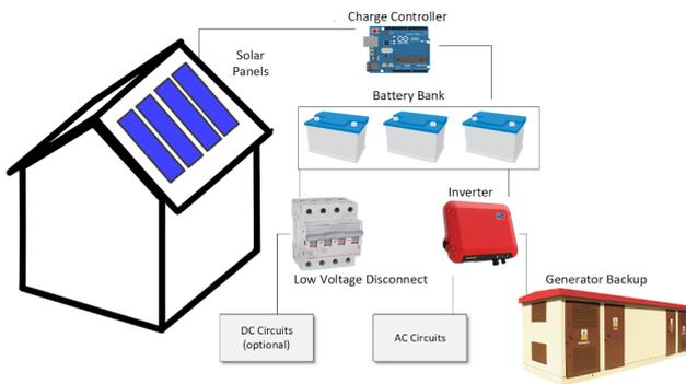
Fig. 2 Off-grid PV System
