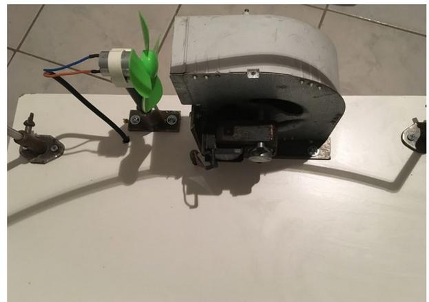
Fig. 6 Mini wind turbine with the inflow providing the source
