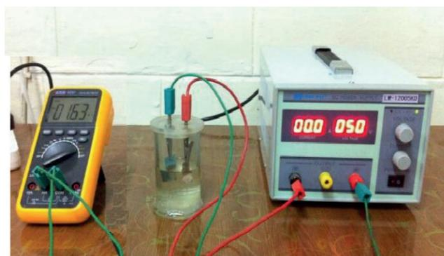
Fig. 1 Instruments of titanium anodization experiment.
