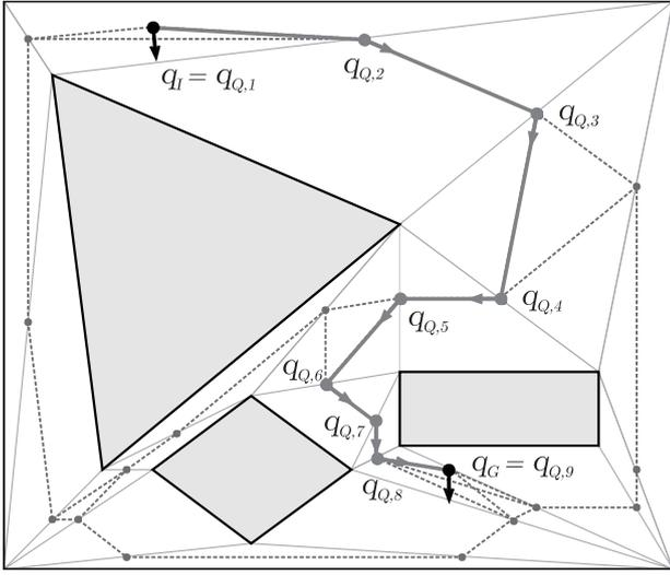
Fig. 4. Preliminary path based on triangular cell decomposition
