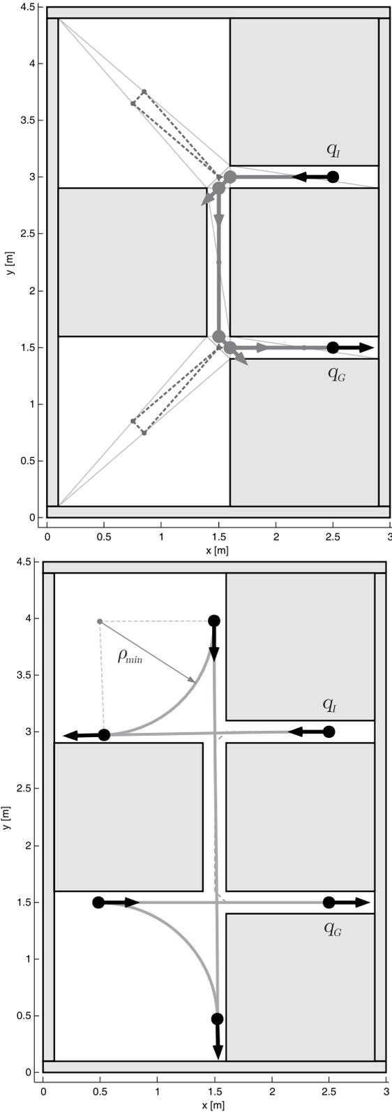
**Fig. 6.** Test scenario 1:  $\min(\eta(q)) = 2.667$ ,  $\eta(\Gamma) = 20$  (a) Cell decomposition, roadmap and preliminary path, (b) Resulting path
