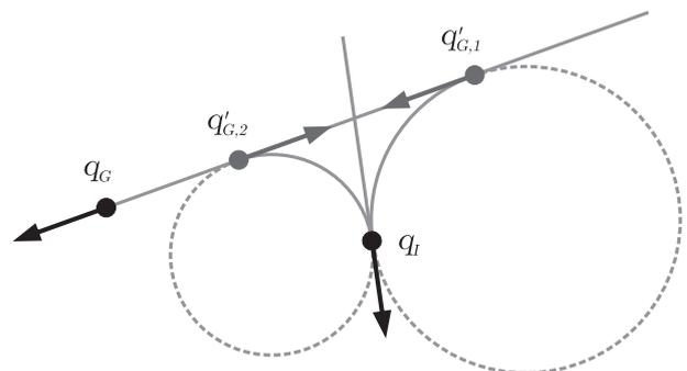
**Fig. 3.** Local *CS* path between two configurations
