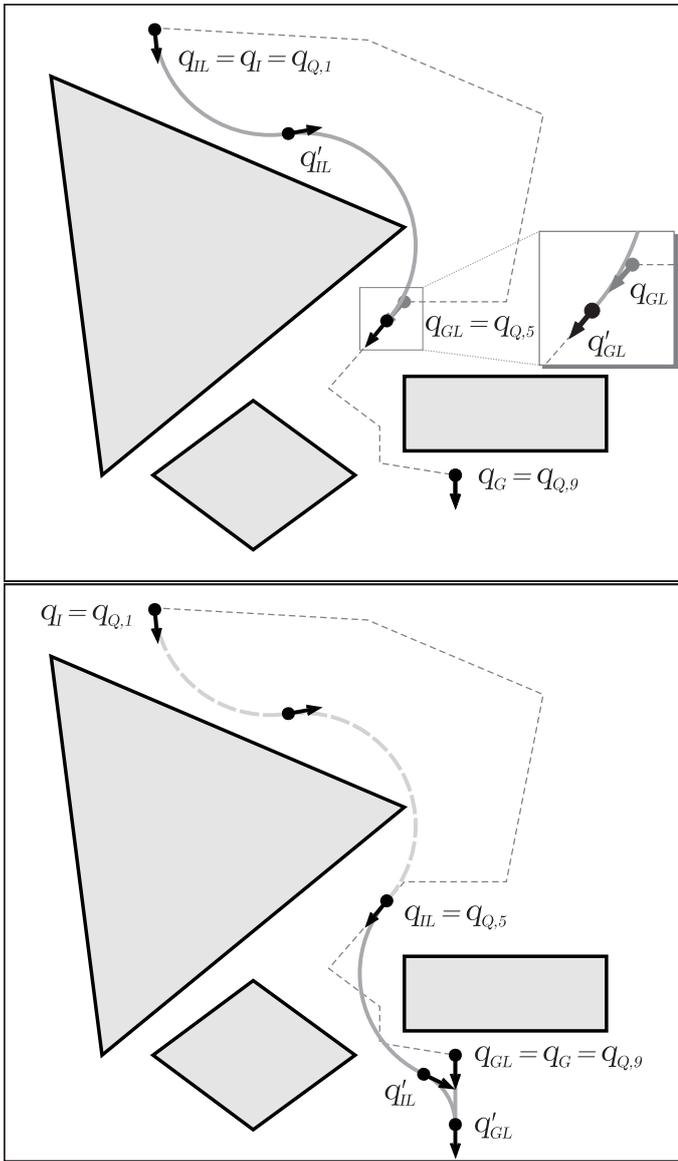
**Fig. 5.** Execution of the planning algorithm (a) Step 1:  $q_{IL} = q_I$ ,  $q_{GL} = q_{Q,5}$ , (b) Step 2:  $q_{IL} = q_{Q,5}$  (updated),  $q_{GL} = q_G$
