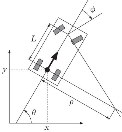
Fig. 1. Model of a car-like robot
