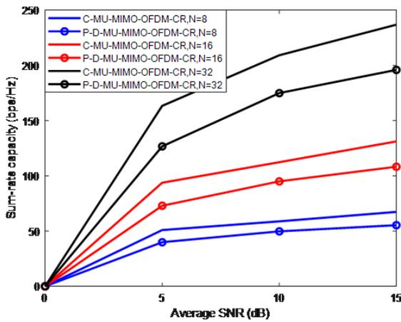
Fig. 2 Sum-rate capacities versus average SNR of C-MU-MIMO-OFDM-CR, and P-D-MU-MIMO-OFDM-CR for different numbers of subcarriers
