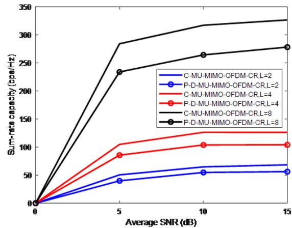
Fig. 4 Sum-rate capacities versus average SNR for C-MU-MIMO-OFDM-CR, and P-D-MU-MIMO-OFDM-CR for different numbers of spatial sub-channels
