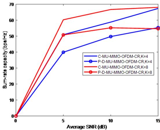
Fig. 3 Sum-rate capacities versus average SNR of C-MU-MIMO-OFDM-CR and P-D-MU-MIMO-OFDM-CR for different numbers of users
