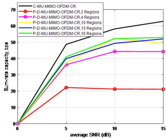
Fig. 5 Sum-rate capacity versus average SNR of P-D-MU-MIMO-OFDM-CR for different numbers of discrete rate levels
