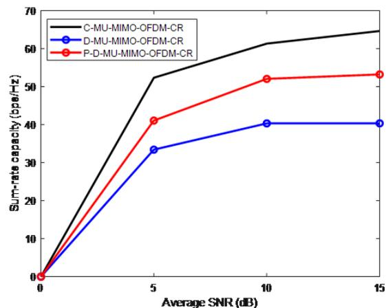
Fig. 1 Sum-rate capacities versus average SNR of C-MU-MIMO-OFDM-CR, D-MU-MIMO-OFDM-CR and P-D-MU-MIMO-OFDM-CR schemes
