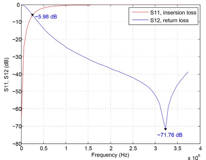
Fig. 10 Insertion and return losses versus frequency
