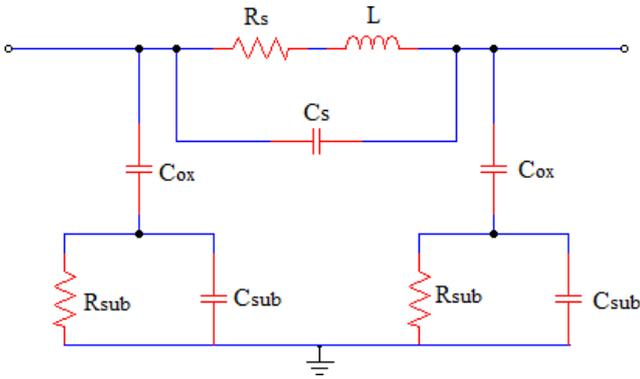
Fig. 4 Equivalent circuit of an integrated inductor
