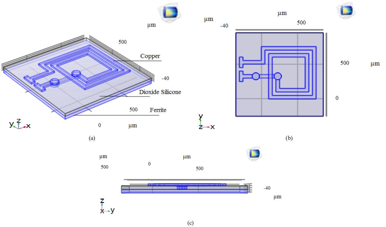
Fig. 3 Magnetic core integrated inductor topography, (a) general view, (b) top view, (c) front view
