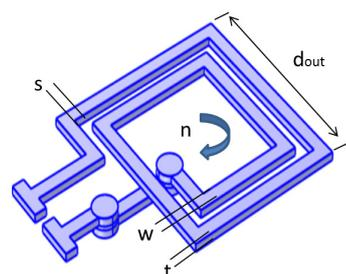
Fig. 1 Geometry of integrated planar spiral inductor
