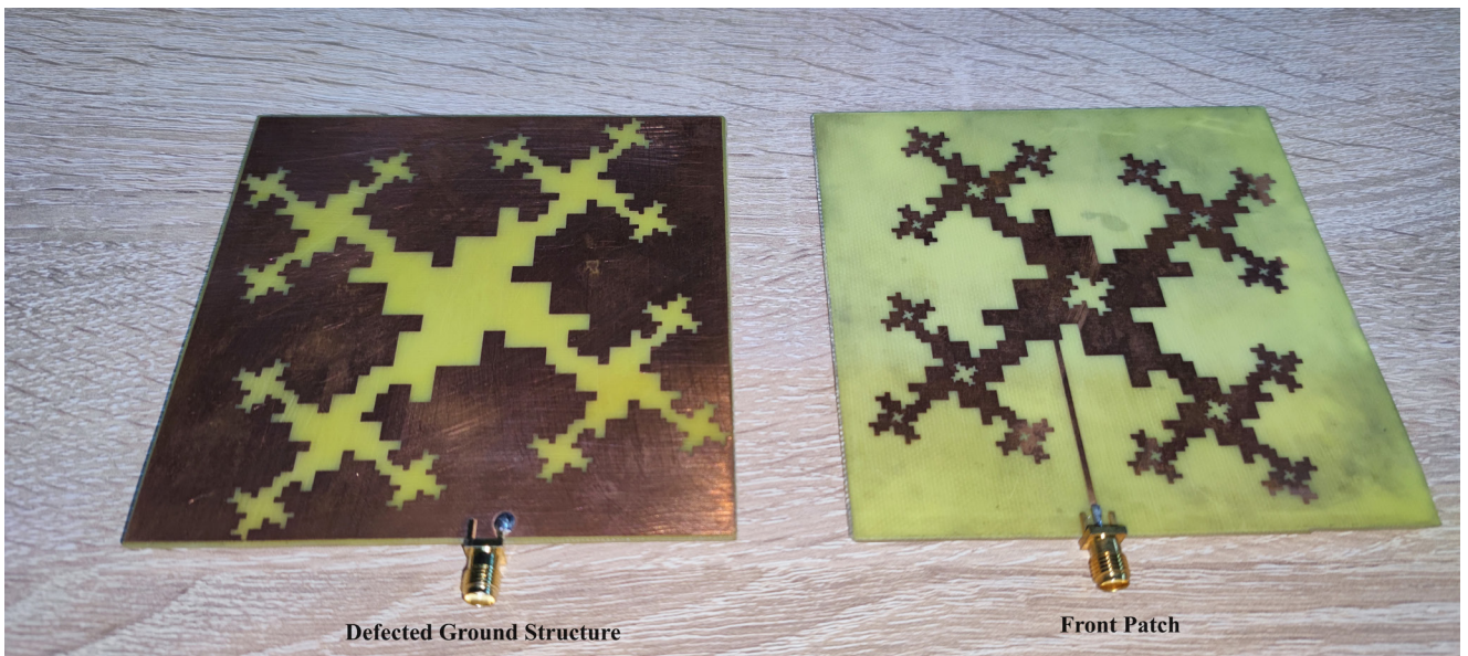
Fig. 15 Photograph of the physical structure of the proposed (Antenna-1-d)
