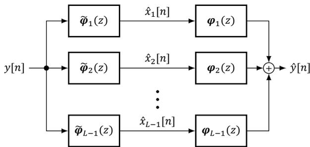
Fig. 8 FIR-based implementation of discrete Gabor transforms
