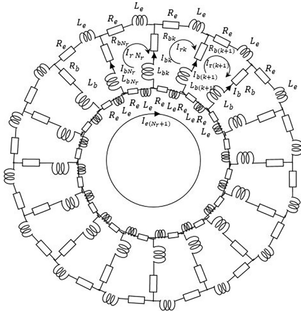
Fig. 1 The equivalent circuit of the rotor squirrel-cage
