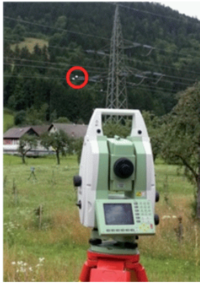
Fig. 10 Measuring station LEICA TS30 (OTLM devices are encircled in yellow)
