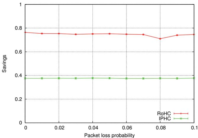
**Fig. 14** Average header savings  $S_h(i)$  attained with RoHC TCP profile and IPHC reference implementations for a radio stream over an IPv4 link containing the TCP acknowledgements (upstream) with different uncorrelated packet loss probabilities.
