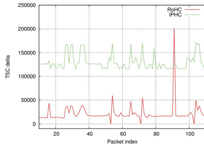
**Fig. 10** Header decompression complexity measured by CPU timestamps (TSC) attained with RoHC TCP profile and IPHC reference implementations for the acknowledgement stream of a digital radio transmission.
