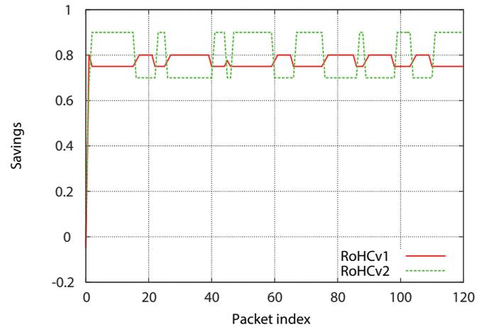
Fig. 6 Header compression savings  $S_H(i)$  attained with RoHCv1 and RoHCv2 RTP profile reference implementations for an IPv4 audio only stream over a reliable unidirectional channel using the RTP profile.
