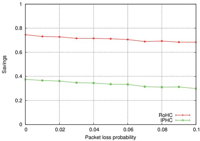
**Fig. 13** Average header savings  $S_h(i)$  attained with RoHC TCP profile and IPHC reference implementations for a radio stream over an IPv4 link containing the audio payload (downstream) with different uncorrelated packet loss probabilities.
