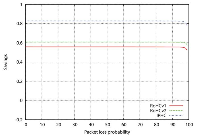
**Fig. 12** Average header savings  $S_H(i)$  attained with RoHC UDP profile and IPHC reference implementations for a UDP stream over an IPv4 link with different uncorrelated packet loss probabilities.
