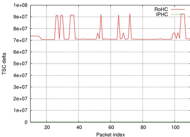
**Fig. 9** Header compression complexity measured by CPU timestamps (TSC) attained with RoHC TCP profile and IPHC reference implementations for the acknowledgement stream of a digital radio transmission.
