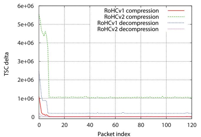
**Fig. 3** Header (de)compression complexity measured by CPU timestamps (TSC) attained with RoHCv1 and RoHCv2 RTP profile reference implementations for VoIP call with GSM full rate codec using IPv4 over WLAN.
