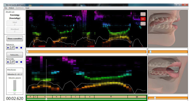
Fig. 1 Practicing user interface of Speech Assistant. 45-degree-angle and 90-degree-angle views of the talking head (right), segmented visual representation of the reference speech (bottom left) and the representation of the speech sound recorded during practicing (top left).
