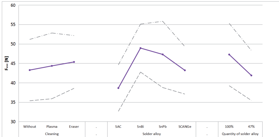
Fig. 9 Influence of factors on the mechanical shear strength from DOE method
