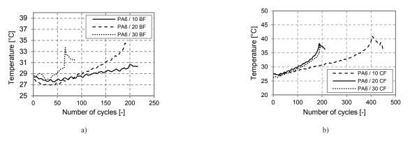
Fig. 3 Temperature of basalt fiber reinforced composites (a) and carbon fiber reinforced composites (b) during fatigue test carried out at 80% of tensile strength
