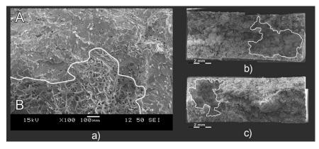
Fig. 5 Fracture surfaces of basalt fiber reinforced composites (a) after fatigue test carried out at 80% (b) and 90% (c) of the tensile strength (tough fracture surface inside the white border)
