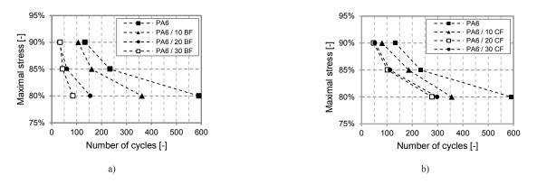
Fig. 2 S-N curve at different load levels: a) basalt fiber reinforced composites, b) carbon fiber reinforced composites
