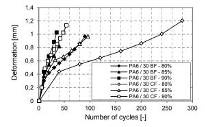
Fig. 4 Cyclic creep of composites with 30 wt% basalt and carbon fiber content at different load levels
