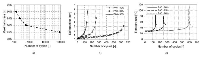
Fig. 1 Polyamide 6 fatigue tests results: a) Stress – Number of cycles curve, b) cyclic creep of the material at different loads, c) temperature of the specimen at different loads
