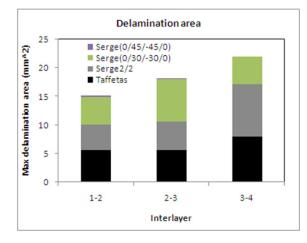
Fig. 7 Maximum delamination area
