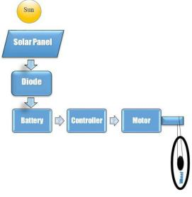
Fig. 1 power generation system for a tricycle.
