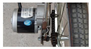
Fig. 2 Power transmission from motor to wheel
