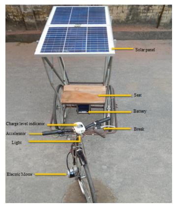
Fig. 4 Experimental view of the tricycle
