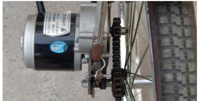
Fig. 2 Power transmission from motor to wheel
