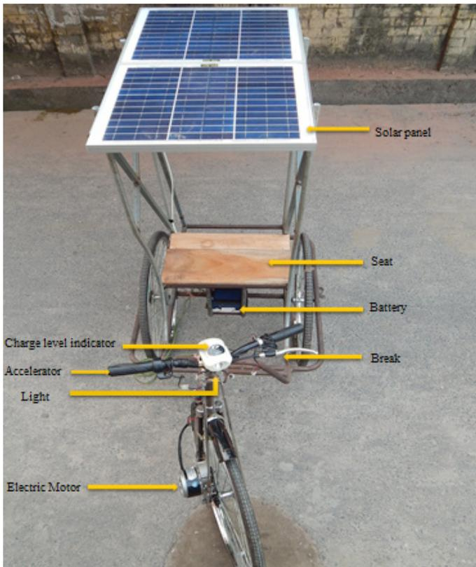
**Fig. 4** Experimental view of the tricycle
