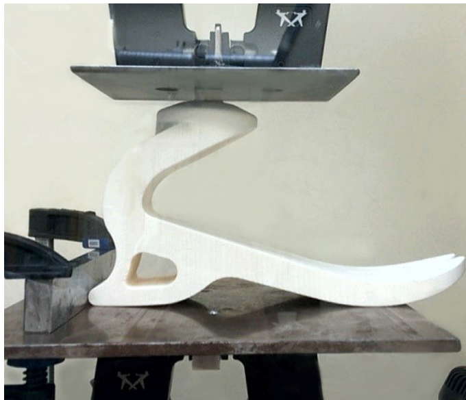
Fig. 3 The compression investigation of the prototype.
