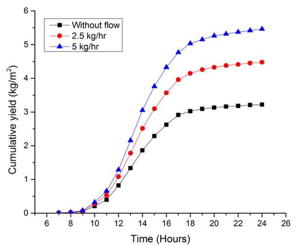
Fig. 9 (a) Variation of cumulative yield from modified solar still with different water mass and constant water flow around the basin
