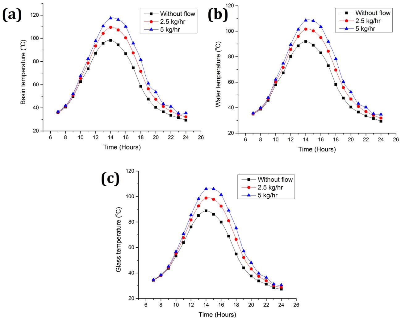
Fig. 6 Hourly variation of (a) basin, (b) water, and (c) glass temperature with different mass flow around the basin and constant water mass ( $m_w = 20$  kg)
