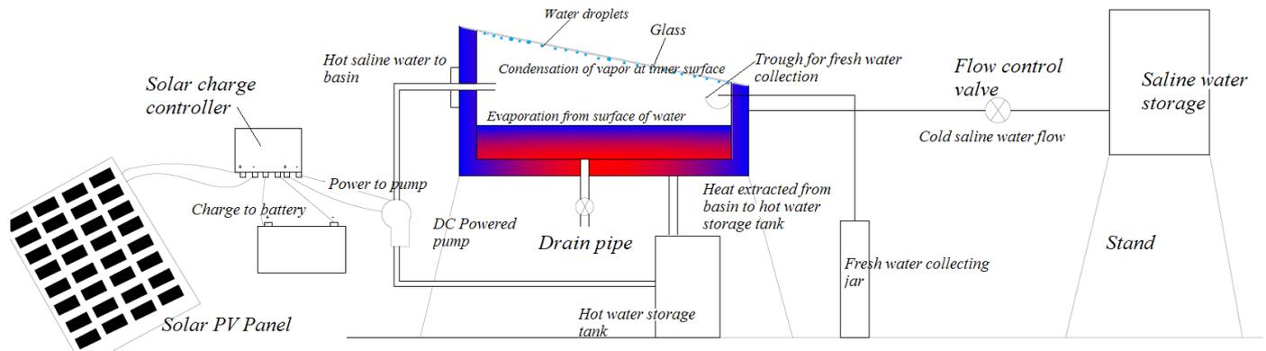
Fig. 1 Schematic diagram of single slope solar still with continuous extraction of heat from basin
