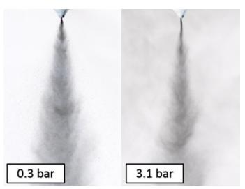
Fig. 4 Spray structure at 0.3 bar (left) and 3.1 bar (right) atomization pressures.
