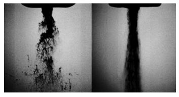
Fig. 5 Atomization at 0.3 bar (left) and 2.4 bar (right) atomizing gauge pressures.
