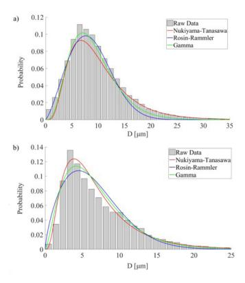
Fig. 6 Three commonly used fitted PDFs at  $p_o = 0.3$  bar. a) z = 10, b) 50 mm.
