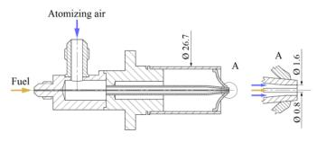
Fig. 1 Cross section of investigated atomizer.
