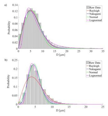
Fig. 9 Four alternative fitted PDFs at  $p_g = 3.1$  bar. a) z = 10, b) 50 mm.
