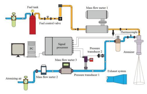
Fig. 3 The measurement configuration.
