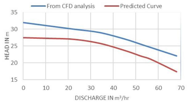
**Fig. 19** Head vs. Discharge
