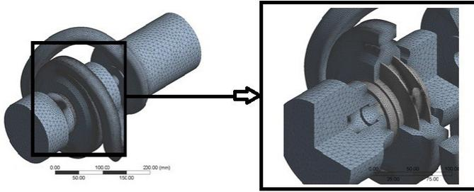
Fig. 12 Meshing of model
