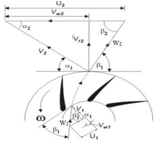
Fig. 4 Inlet and outlet velocity triangle
