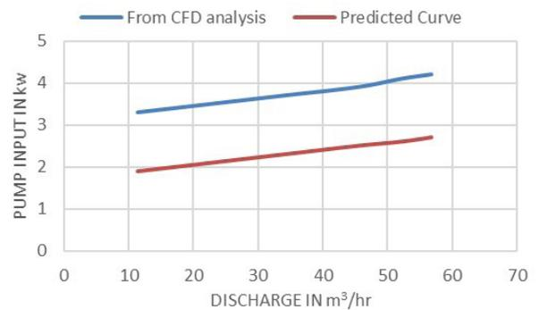
**Fig. 21** Pump Input vs. Discharge
