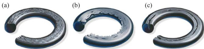
Fig. 2 Typical failure of O-rings. (a) Excessive wear, (b) Extrusion, (c) Excessive initial compression [6].
