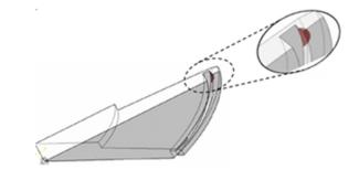
Fig. 4 Semi elliptical crack at blade mounting location
