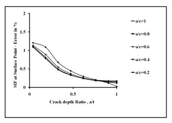
Fig. 9 Error- Stress Intensity Factor at surface Point
