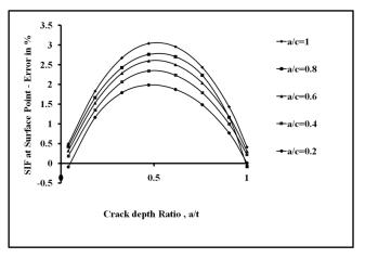
Fig. 10 Error- Stress Intensity Factor at deepest Point
