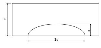
Fig. 3 Semi Elliptical Crack
