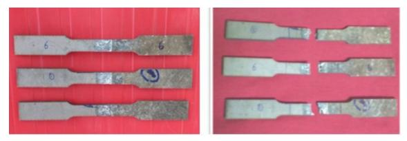
Fig. 5 Tensile Specimen of Dissimilar Alloys
