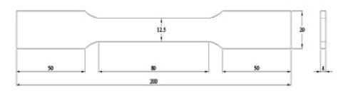
Fig. 4 Tensile Specimen with ASTM E8M
