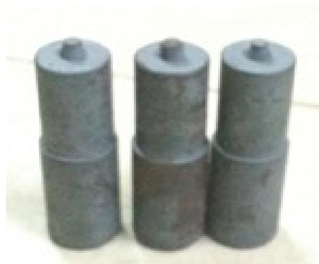
Fig. 2 Tool after Hardening
