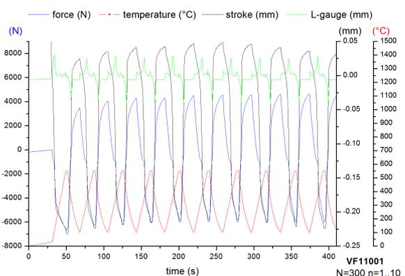
Fig. 8. Thermal-fatigue simulation results of 15Mo3 material versus time (0 – 10 cycles).
