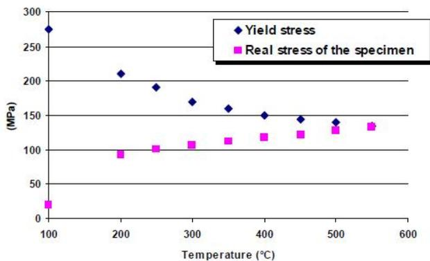
Fig. 11. Compression stress in the specimen during the stress versus temperature.
