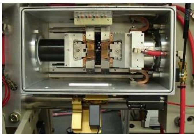
Fig. 2. Work chamber of Gleeble 3800 [7]
