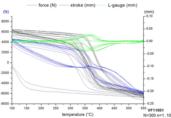
Fig. 9. Thermal-fatigue simulation results of 15Mo3 material versus temperature.
