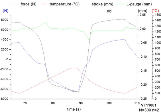
Fig. 10. Second cycle of the 15Mo3 thermal-fatigue simulation.
