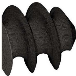
Fig. 6. A thickened finite element net at the end of the screw.
