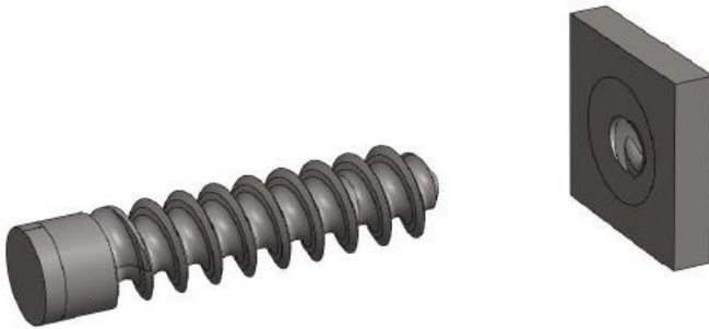
Fig. 2. The initial geometric model (prism-shaped bone model.)
