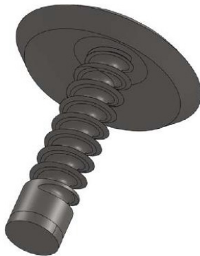
Fig. 3. The screw for the neck of the femur in a screwed – in position in the subchondral layer (spherical calotte model.)
