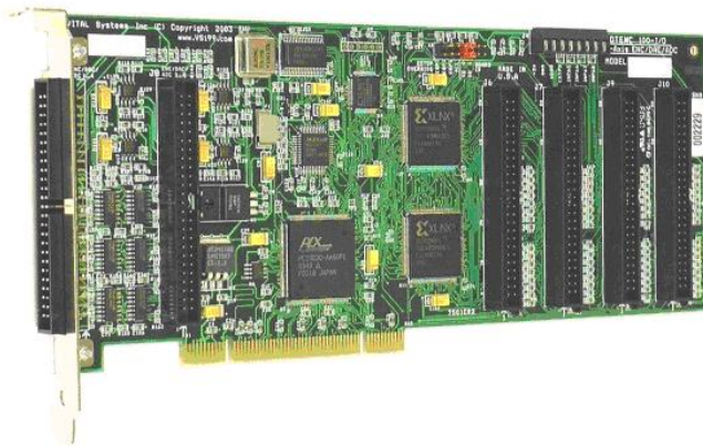
Fig. 2. Vital System's 8-Axis Motion Control & Data Acquisition PCI Board
