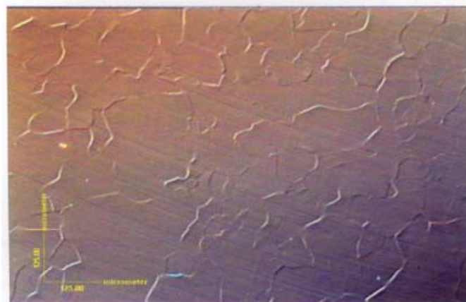
Fig. 1. Microcut surface by microscope (500X)
