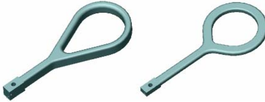
Fig. 6. Initial and optimal shape of handhold
