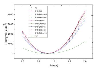
Fig. 4 Variation of the J-integral along the thickness of FGM plate for a normalized crack length. Mode I + II + III
