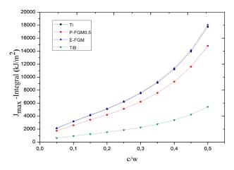
**Fig. 6** Variation of the maximal J-integral according to cracknormalized length emanating from the notches. Mode I + II + III
