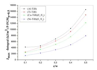
Fig. 12 Variation of the maximal J-integral according to normalized length emanating from notches for various Young's modulus of ceramic. Mode I + II + III
