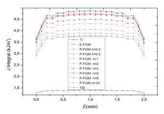
Fig. 3 Variation of the J-integral along the thickness of FGM plate for a normalized crack length. Mode I
