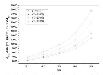
Fig. 16 Variation of the maximal J-integral according to normalized length emanating from notches for various applied loading. Mode I + II + III
