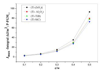
Fig. 13 Variation of the maximal J-integral according to normalized length emanating from notches for various Young's modulus of metal. Mode I
