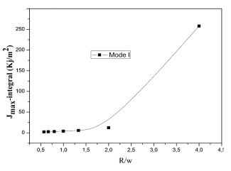
Fig. 10 Variation of the maximal J-integral according to normalized length emanating from notches for versus notch radius for Ti-TiB plate with P-FGM) n = 0.5. Mode I + II + III
