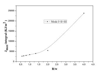
Fig. 9 Variation of the maximal J-integral according to normalized length emanating from notches for versus notch radius for Ti-TiB plate with P-FGM) n = 0.5. (a) Mode I
