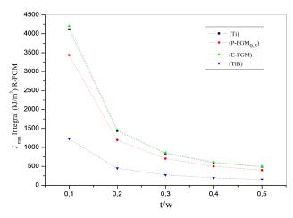
Fig.8 Variation of the maximal J-integral according to the various normalized thickness. Mode I + II + III
