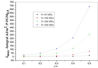
Fig. 15 Variation of the maximal J-integral according to normalized length emanating from notches for various applied loading. Mode I
