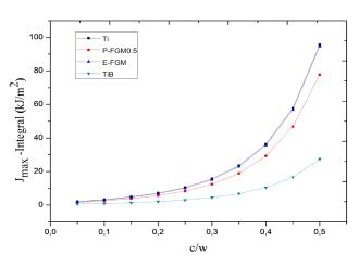
Fig. 5 Variation of the maximal J-integral according to cracknormalized length emanating from the notches. Mode I
