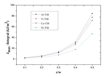
Fig. 11 Variation of the maximal J-integral according to normalized length emanating from notches for various Young's modulus of ceramic. Mode I
