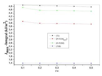
Fig. 7 Variation of the maximal J-integral according to the various normalized thickness. Mode I
