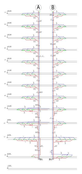
Fig. 5 Scheme of risers A and B  $(BV_A, BV_B - balancing valves Danfoss MSV BD)$
