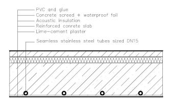
Fig. 1 Detail of the CRITTALL ceiling system
