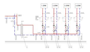
Fig. 3 Heat distributor of 1st pressure zone
