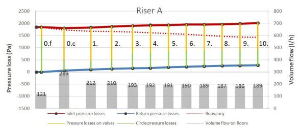
Fig. 8 Pressure diagram and volume flow distribution of riser A by temperature drop 35/30.5°C
