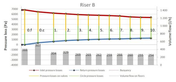
Fig. 11 Pressure diagram and volume flow distribution of riser B by temperature drop 25/25°C
