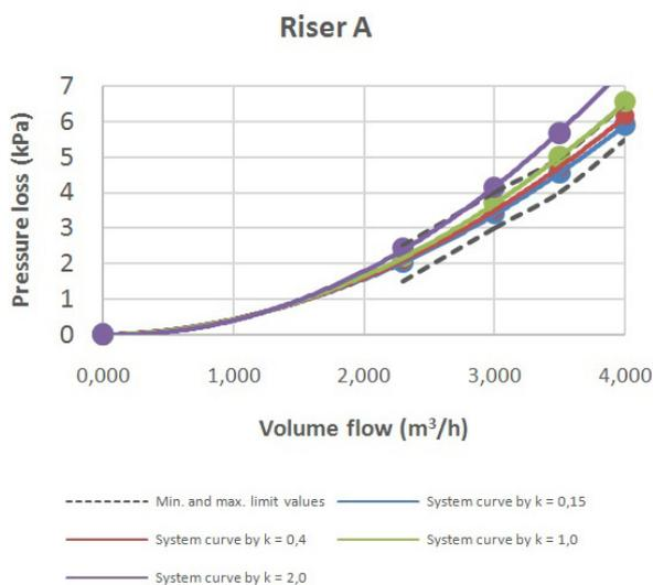
Fig. 6 Comparison of characteristic curves of risers A by various reference roughness with measurements data (by reference mean fluid temperature 25 °C)
