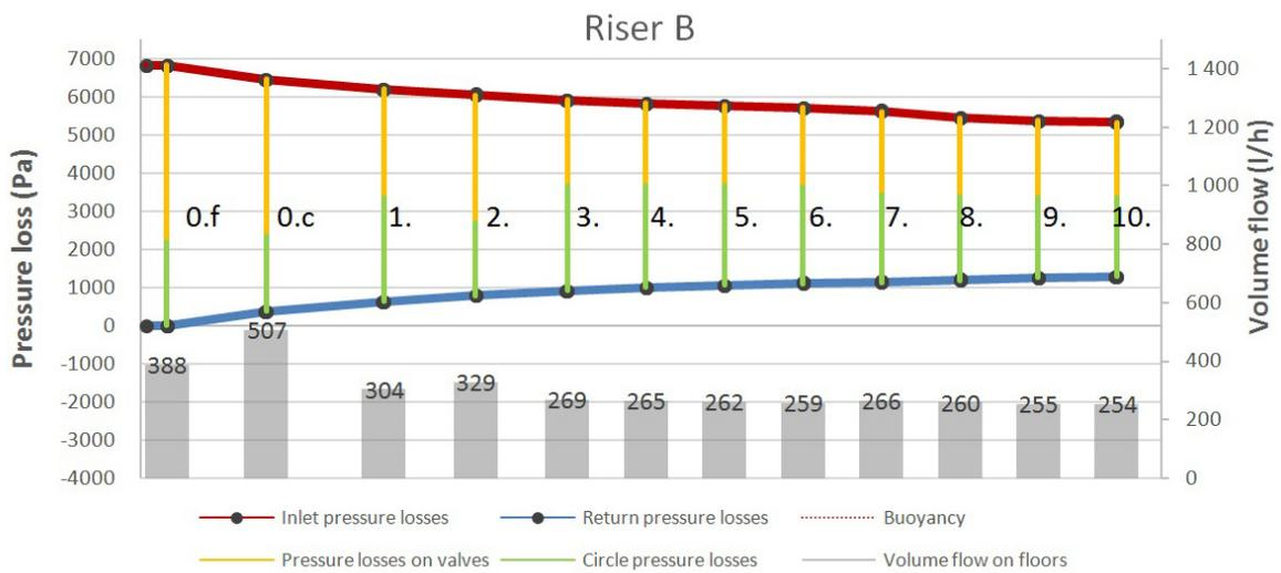
Fig. 10 Pressure diagram and volume flow distribution of riser B by temperature drop 35/31.5°C
