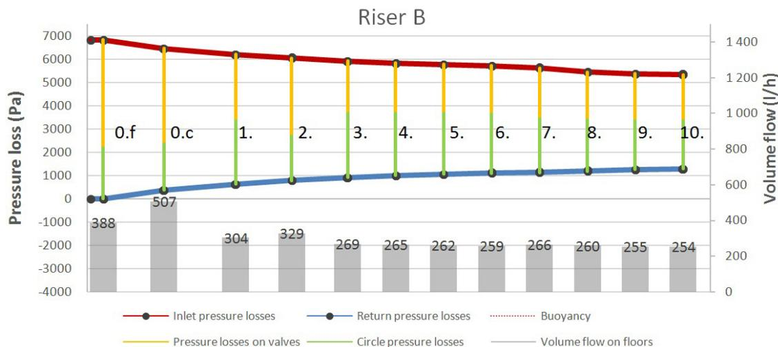
Fig. 11 Pressure diagram and volume flow distribution of riser B by temperature drop 25/25°C
