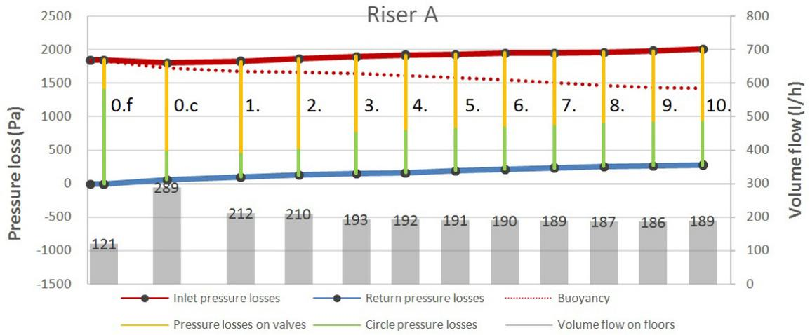
Fig. 8 Pressure diagram and volume flow distribution of riser A by temperature drop 35/30.5°C
