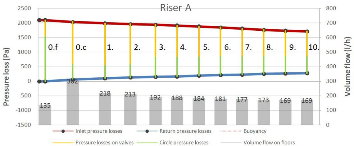
Fig. 9 Pressure diagram and volume flow distribution of riser A by temperature drop 25/25°C
