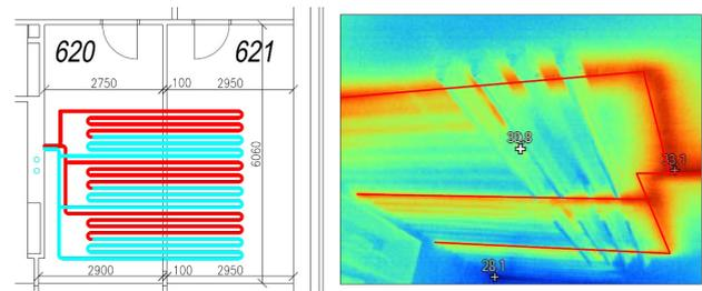
Fig. 4 Heating pipes in ceiling determined by thermocam (1 – hydraulic separator, 2 – circulator pump, 3 – three-way mixing valve)
