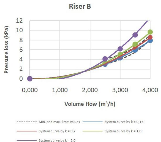
Fig. 7 Comparison of characteristic curves of risers B by various reference roughness with measurements data (by reference mean fluid temperature 25 °C)
