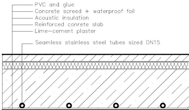
Fig. 1 Detail of the CRITTALL ceiling system
