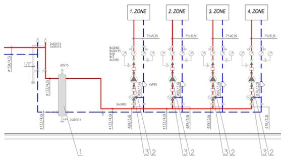
Fig. 3 Heat distributor of 1<sup>st</sup> pressure zone
