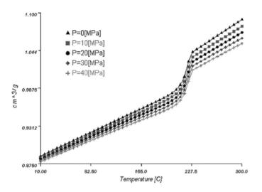
*Fig. 1.* The specific volume vs. temperature (pvT) curves for PA6 (Bayer Durethan B 30 S)
