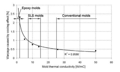
Fig. 5. The influence of the mold thermal conductivity on warpage
