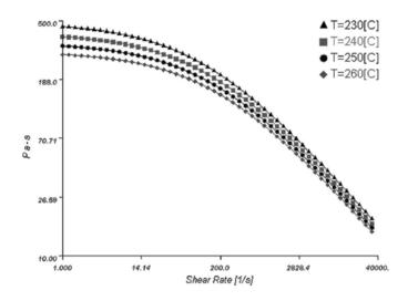
*Fig. 2.* Viscosity – shear rate function for PA6 (Bayer Durethan B 30 S)
