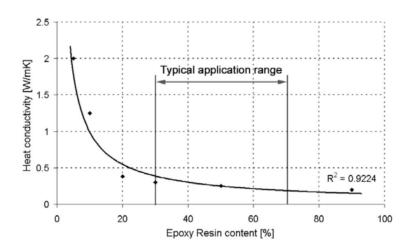
*Fig. 4.* Heat conductivity of metal powder filled epoxy
