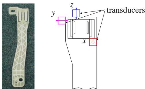
*Fig. 1.* Junction box bracket. The bottom part is fixed to the car body while the top part holds the actual box. In our measurements, the bottom part is fixed to the jarring table while accelerations are measured at the indicated positions.
