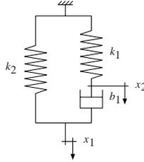
Fig. 6. Three-parameter Maxwell model
