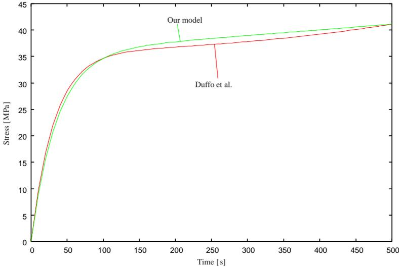
Fig. 4. Material law fitting (at  $\dot{\varepsilon} = 10^{-3} \frac{1}{\text{s}}$ )
