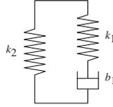
Fig. 3. Three-parameter Maxwell model
