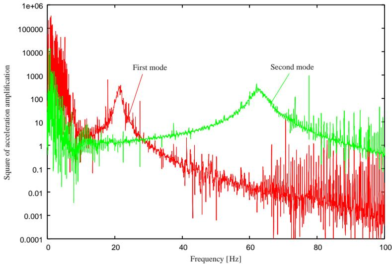
Fig. 2. Measurement results. The first mode is a bending vibration (excitation and accelerometer along  $x$ ), while the second one is torsional (excitation and accelerometer along  $y$ ).
