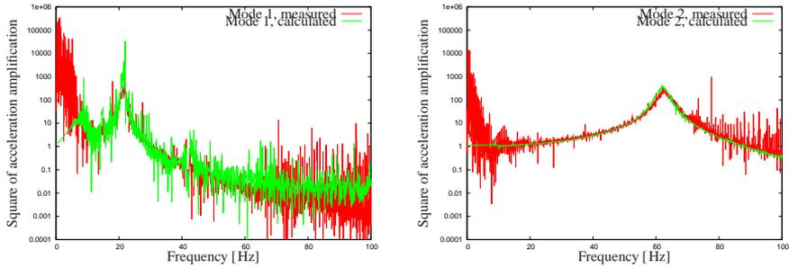
Fig. 5. Measured and calculated transfer functions for modes 1 and 2.
