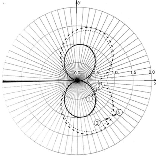
Fig. 4. The shape of the plastic zone around the crack tip in plane strain calculated basing on the 'conical' theory for the working stress. 1.  $\Psi = 0.8$ ,  $\nu = 0.36$ ; 2.  $\Psi = 0.8$ ,  $\nu = 0.5$ ; 3.  $\Psi = 0.5$ ,  $\nu = 0.36$ ; 4.  $\Psi = 0.5$ ,  $\nu = 0.5$ .
