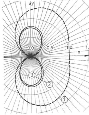
Fig. 2. The size of the plastic zone around the crack tip presented in dimensionless form  $r/\Phi$  calculated applying the von Mises working stress. 1. Plane stress; 2. Plane strain with  $\nu = 0.36$ ; 3. Plane strain with  $\nu = 0.5$ .
