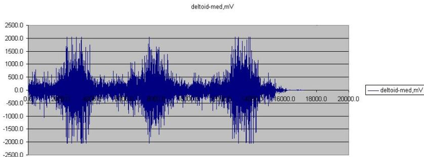
Fig. 7. Muscle activity measurement results, EMG curves
