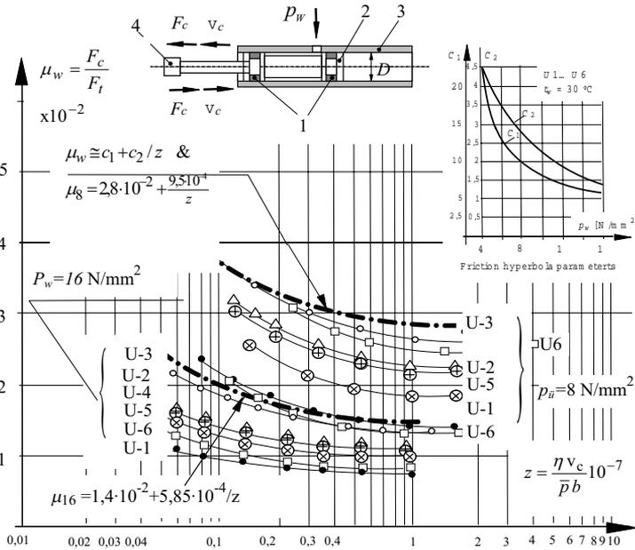
Fig. 7. Friction coefficient ('Stribeck') diagrams of Polyurethane U-rings (having different shapes in the same cross section)<sup>(2)</sup>
