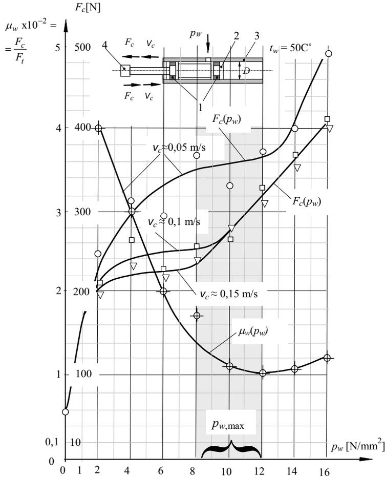
Fig. 4. Friction force – working pressure and friction coefficient – working pressure diagrams of Silicon U-rings<sup>(1)</sup>
