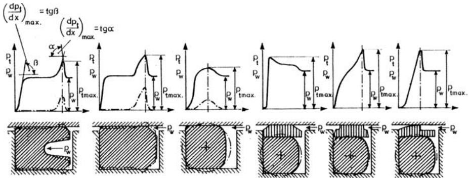
Fig. 3. Static sealing pressure distribution profiles of some reciprocating hydraulic seals having single friction edges. (From left to right: Elastomeric U-ring,  $\square$ -ring, O-ring and compact composite seals with O-ring and different reinforced PTFE piston rod seal.)
