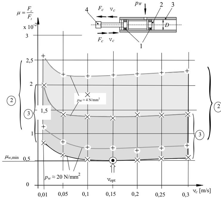
Fig. 6. Friction coefficient – reciprocating speed diagrams of Polyurethane U-rings (2) and NBR O-rings (3)<sup>(2)</sup>
