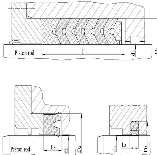
Fig. 2. Seal housings for hydraulic piston rods
