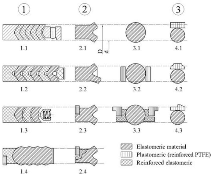
*Fig. 1.* A typical classification of reciprocating hydraulic seals
