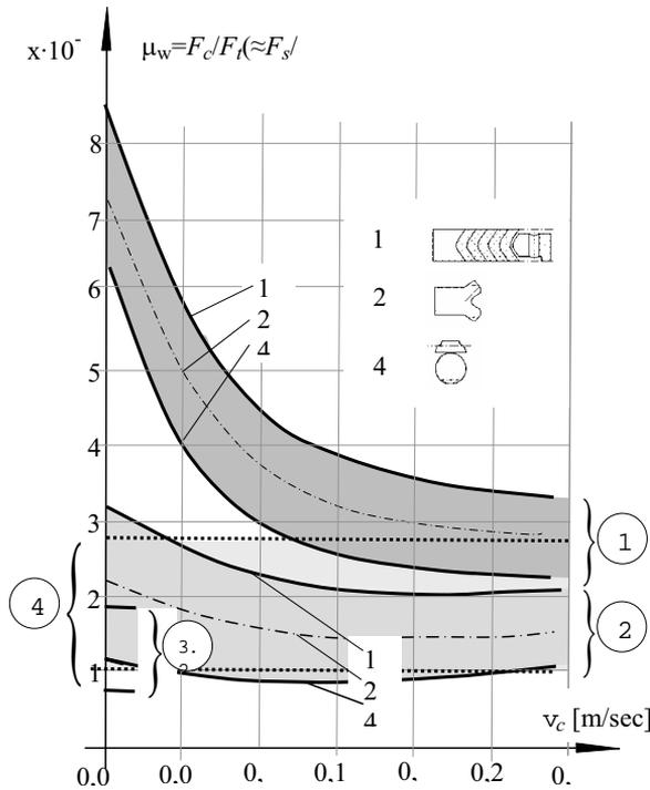
Fig. 9. Friction coefficient in the function of reciprocating speed for hydraulic piston seal<sup>(2)(4)(5)</sup>
