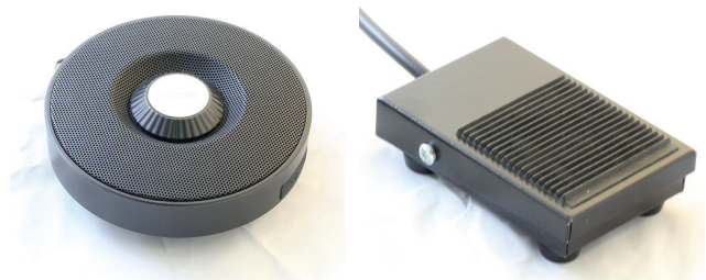
Fig. 12 Left: Peripheral unit for sound stimulus, right: Pedal peripheral unit for reaction detection
