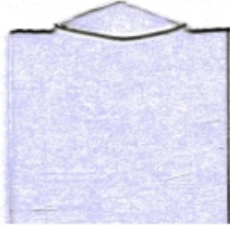
Fig. 4. Light microscopic picture taken on the necked ligament of a DDEN-T specimen of COP 68 with l = 20 mm
