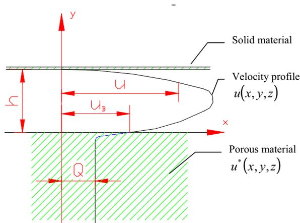
Fig. 1. The torn velocity profile in oil film
