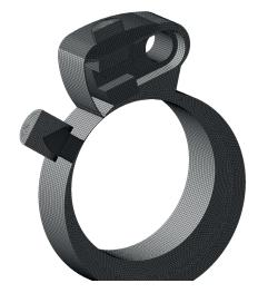
Fig. 9 Mesh of the computational domain, including only prismatic elements within the dynamic mesh domain
