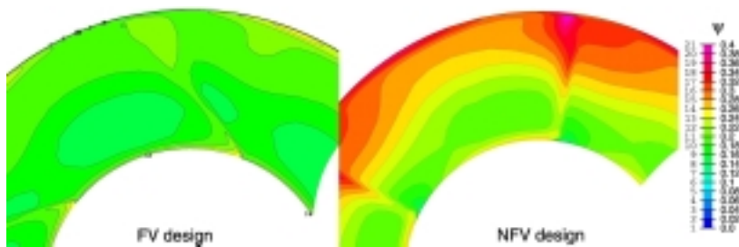
Fig. 6. \psi local flow coefficient distribution downstream of the rotors on a plane perpendicular to rotor axis. Axial distance of the plane is 23 percent of tip diameter from the blade stacking line.
