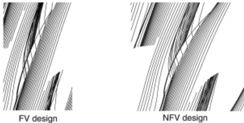
Fig. 7. Streamlines approaching the blades at the mid-radius of tip clearance
