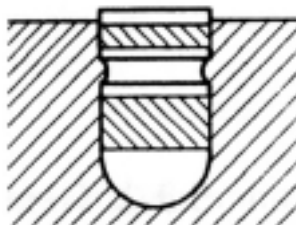
Fig. 2. Metal insert into polymer element to join metric bolts
