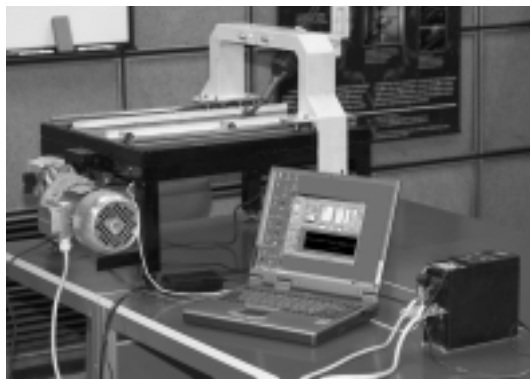
Fig. 6. Computer controlled hot-air-blowing welding device
