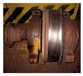
Fig. 8 An inappropriate wear and tear of the running wheel flange of the crane
