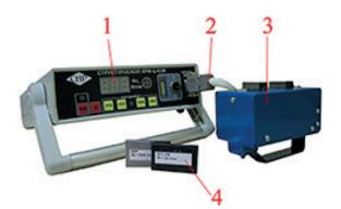
Fig. 1 The exterior of the KRM-CK-2M device: 1 – measuring block; 2 – connecting cable; 3 – transformer; 4 – control samples
